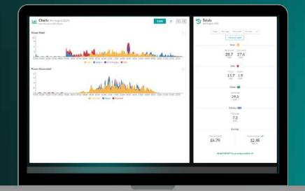
The Powervault Portal incorporates a live view, daily totals and charts that show each 24 hour period. Customers can use scheduling features in the Portal to take advantage of Time of Use (ToU) tariffs. and can optimise their P5 with SMARTSTOR<sup>™</sup>, Powervault's proprietary artificial intelligence energy optimisation system.
